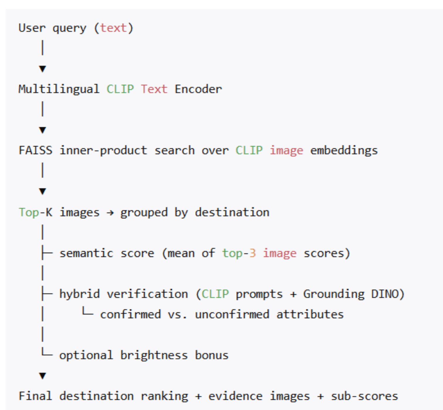
Figure 1. Two-stage retrieval pipeline: semantic search (FAISS over CLIP) + hybrid attribute verification.
